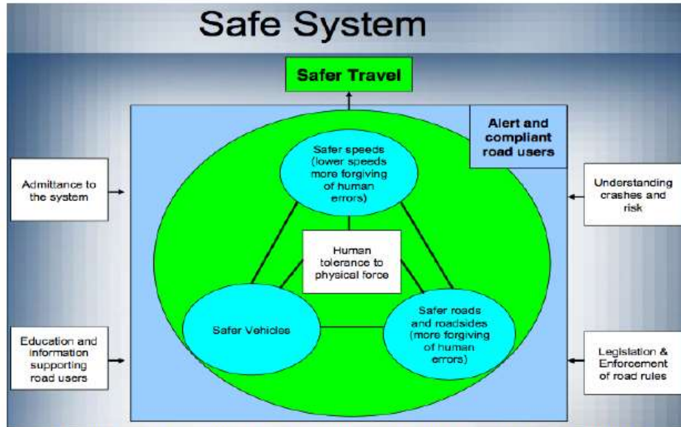
Figure 3 – The Safe System model reproduced from Howard, 2004 [25]
