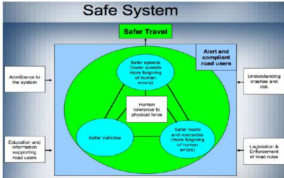
Figure 3 – The Safe System model reproduced from Howard, 2004 [25]
