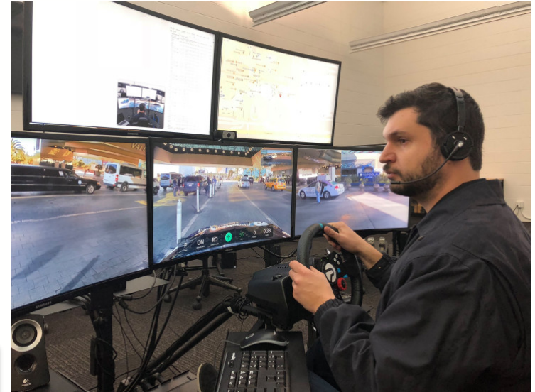
Example of Remote AV Teleoperation, Photo Credit: Phantom Auto (Dickey 2018)
