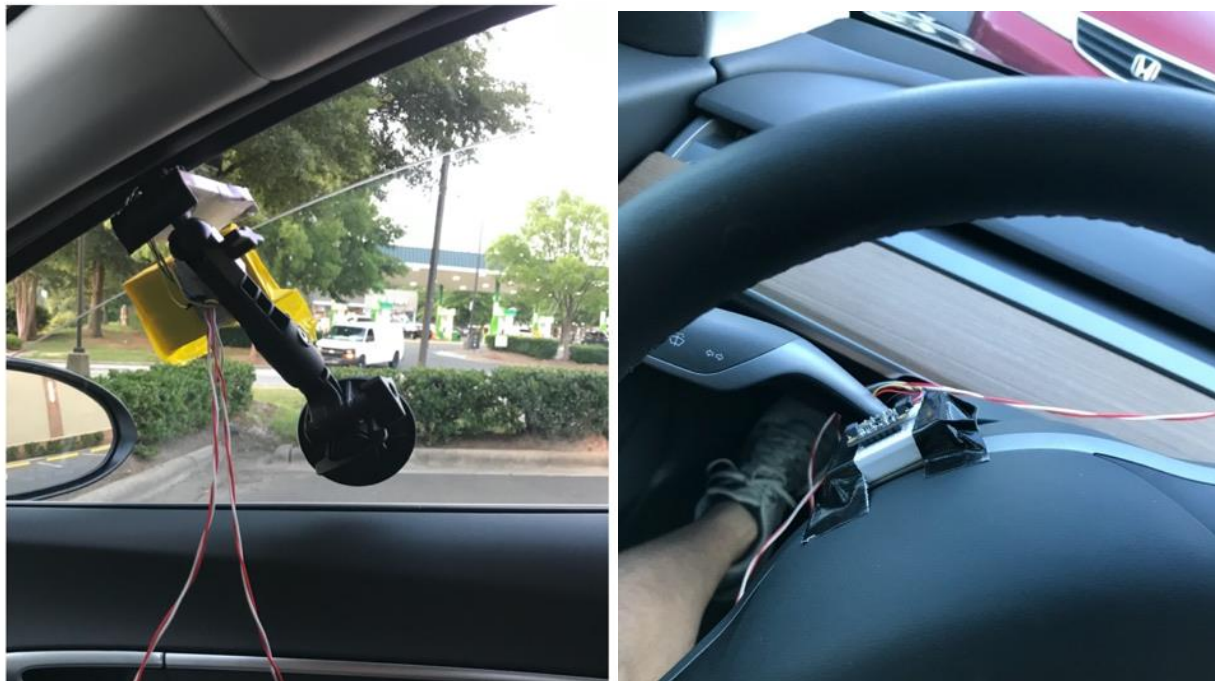
Figure 5: Sensor components. Left: ambient light sensors. Right: acceleration and rotation sensor
