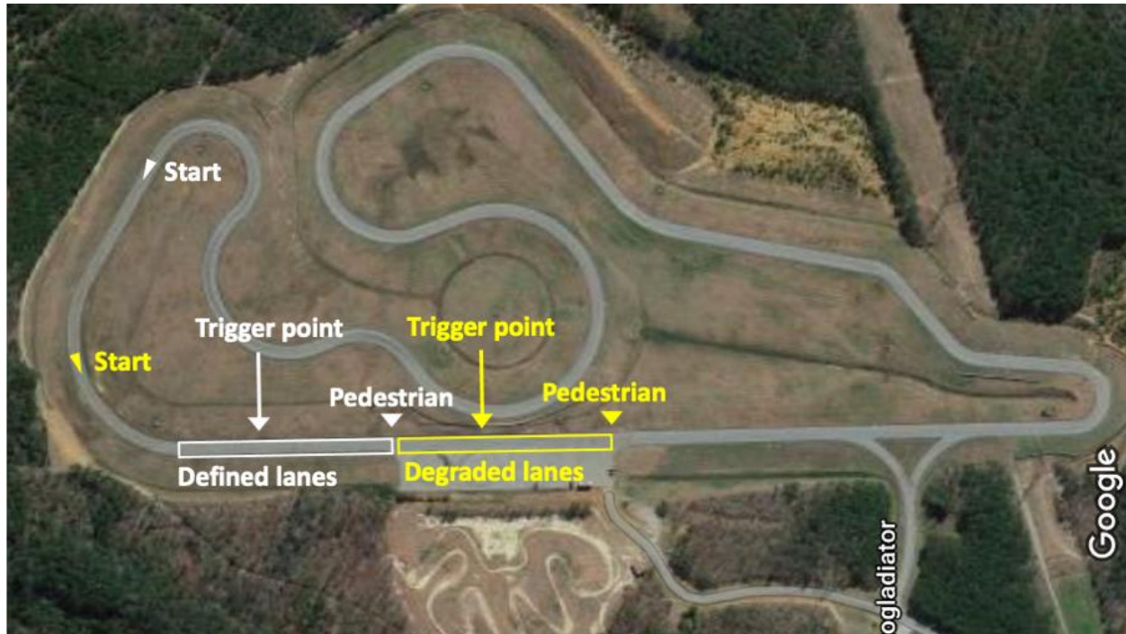
Figure 2: Pedestrian test environment. Defined lanes are marked in white and the degraded lanes condition are marked in yellow.
