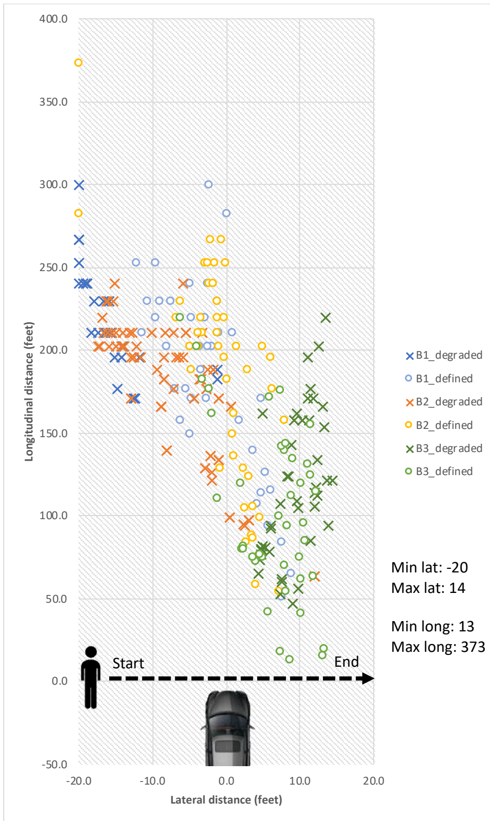
Figure 13: Relative position of pedestrian target to vehicle when pedestrian icon appeared in Model B console
