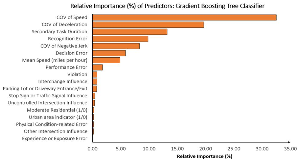
**Figure 8: Feature Importance Plot for the GBT Classifier**
